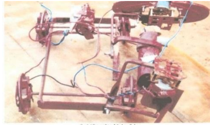
Framework of Paddy Field paring machine
