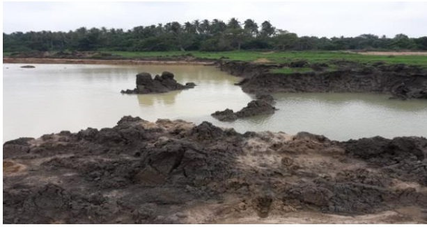
Photographs 13- Soil had been improperly removed for extraction of sand in the Bogoda Lake
